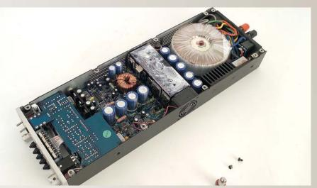
The Briefcase's interior is a model of space efficiency. Note the heatsink tunnel and fan, which separates the sensitive preamp components from the power supply at the rear.
